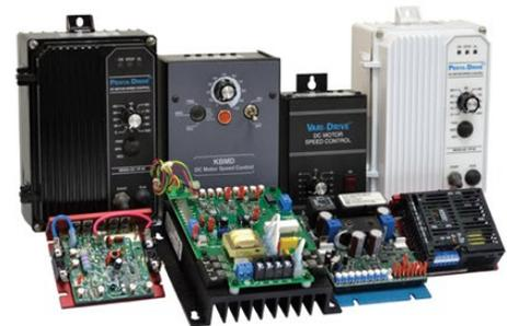
KB standard off-the-shelf DC Drives provide variable speed for DC motors from sub-fractional to 5 horsepower.\* They are available in 115 and 208/230 VAC-50/60 Hz with 1Ø input. Enclosure types include Chassis / IP20, NEMA 1 / IP50 and NEMA 4X / IP65. The NEMA 4X / IP65 drives are housed in a rugged die-cast aluminum enclosure with a hinged cover.
